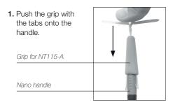
2. To remove the tabs. hold the grip and pull them out. Use a pliers if necessarv.
