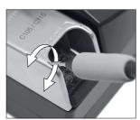
Use the holes to rotate the cartridges for a proper alignment.
