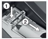
Place the cartridge in the slot as shown and pull the handle to remove it.
