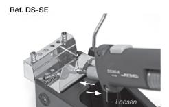
Place the Soldering Iron in the extractor and remove the tip.
