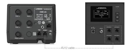
Connect up to 4 stations directly to a fume extractor through the Soldering Station Robot port. Every tool connected to a station can control the aspiration system, but previously it has to be assigned to the fume extractor through the Peripherals menu of the station. Each station detects a fume extractor as a FAE a.
