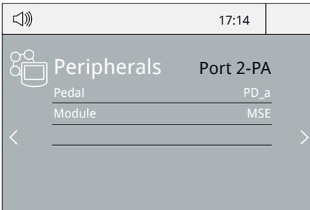
2. Select the pedal from the list (*Note that your first connection is denoted as "a", the second being "b", etc. (e.g. PD\_a, PD\_b,...).*)
