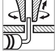
Remove the tip while maintaining the suction to make sure all the solder is removed from the joint.
