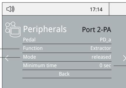
Set the duration of the activation time when pressing the pedal **once\*\***. For continuous functioning keep the pedal pressed.
