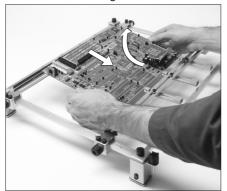
Loosen one sliding guide, pull back and lift out the PCB.
