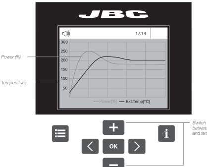
Switch Y axis between power and temperature
