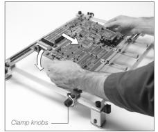
Position it and tighten the sliding guide knobs.
