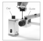
1. Remove both guides by untightening the 8 screws.
